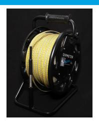
In operation, the probe is lowered down the open bore until it becomes into contact with the water surface. This completes the circuit and activates an alarm. The operator then reads the depth of the probe off the tape at the collar. The probe features a sensitive control to eliminate false water level readings due to dripping water.
