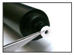
The reference protection ring can be removed and/or replaced (with the electrode still in place in the sensor) by unscrewing the plastic shroud on the end of the electrode. The white protection ring can be slid o the platinum electrode.
