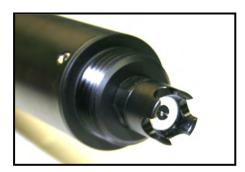
The sensor may be cleaned using a soft cloth, mild detergents and warm water. If the sensor shows signs of marine growth a light biocide can be used to clean and kill any biological growth on the sensor. Sensors are supplied with a removable shroud that provides added protection for the electrode. This shroud unscrews for cleaning.
