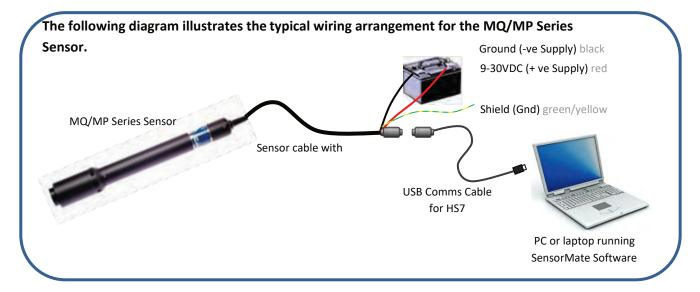
The SensorMate software provides for configuraĆo of the data logger, collection of logged data, and all other functions. For further information, please refer to the SensorMate User Manual.
