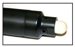
The MQ/MP sensor (with pH or ORP) is shipped with a rubber cap covering the electrode. This cap contains a small amount of 3M KCl solution and is in place to prevent the electrode from drying out during shipping and storage. **This cap must be removed prior to installation.** The cap should be retained so that it can be placed back on the electrode if the sensor is to be removed.
