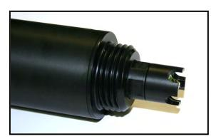
The sensor must be cleaned with the electrode in place. The sensor will be damaged by the ingress of water or other solutions into the electrode cavity. The electrode should only be removed when it is to be replaced. To assist in cleaning the glass electrode, the sensor is provided with a special tool. A few drops of a mild detergent can be placed in the cleaning tool which is then pushed over the glass pH bulb. Carefully rotating the tool by hand should
