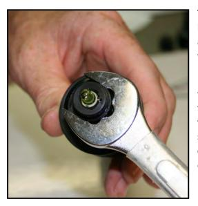
Take care when handling the pH electrode, that it is not handled by the gold contacts. Contamination of this area may degrade the performance and expected life of the electrode
