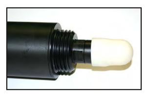
PH electrodes should be stored in such a way to prevent the electrode from drying out. A rubber cap is provided with the electrode for this purpose. A small amount of liquid should be placed in this cap prior to the cap being placed over the electrode. 3M KCl is the preferred storage solution however; tap water should be used if not available. Soaking in pH 4 buffer solution overnight may restore some electrodes that have been allowed to dry out,
