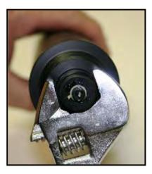
ORP electrodes will require periodic replacement. How long they last is dependent on the environment and to a lesser extent the cleaning and maintenance. In a typical environment, electrode life between 1 and 3 years is quite possible. The electrode is sealed in its mount with two O-rings on the electrode body. The electrode is removed by unscrewing it from the housing. Spanner ats are machined on the electrode to assist.
