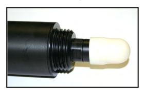
ORP electrodes should be stored in such a way to prevent the electrode from drying out. A rubber cap is provided with the electrode for this purpose. A small amount of liquid should be placed in this cap prior to the cap being placed over the electrode. 3M KCl is the preferred storage solution however; tap water should be used if not available. Soaking in 3M KCl solution overnight may restore some electrodes that have been
