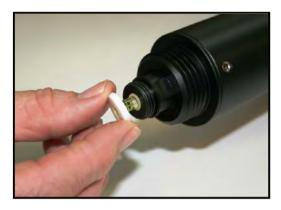
The reference protection ring can be removed and/or replaced (with the electrode still in place in the sensor) by unscrewing the plastic shroud on the end of the electrode. The white protection ring can be slid o the glass electrode.
