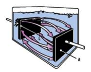
Conductivity can be measured from first principles by using a conductivity cell. This is a box containing a liquid, with two plates, each of area A separated by a distance L.
