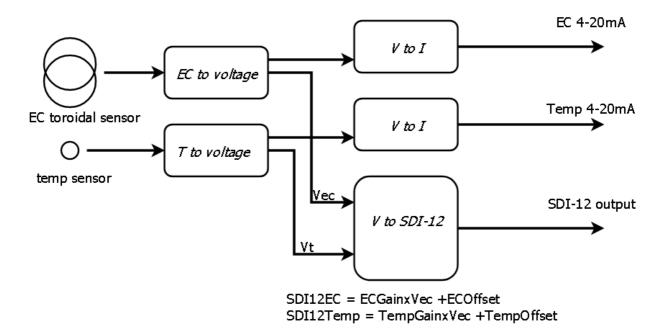
A block diagram of the EC1550 is shown above.
