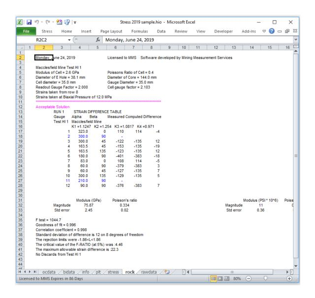
The calculated Modulus and Poisson's ratio are also placed in the info sheet column 2, in rows 37 and 38 respectively.
