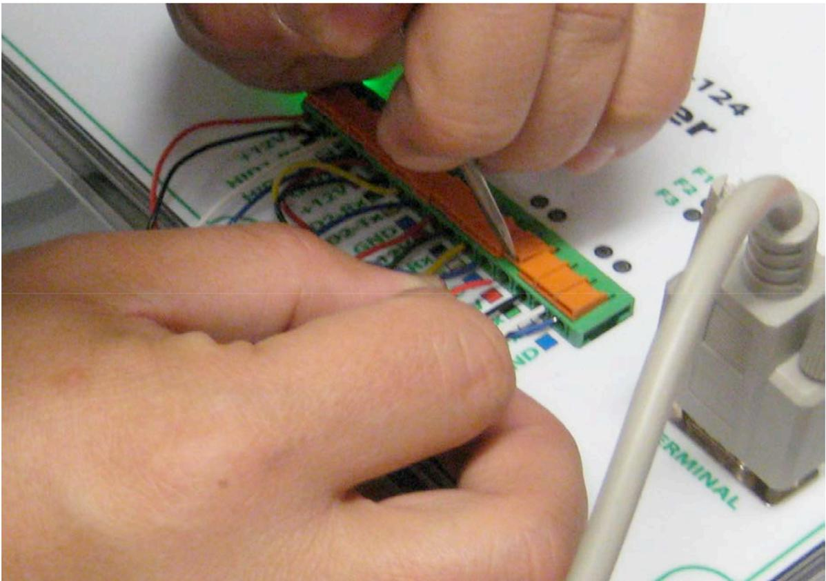
The connectors are designed for use in the field to allow quick and reliable connections. Use a small screwdriver to open the connector while inserting the cable as shown above.
