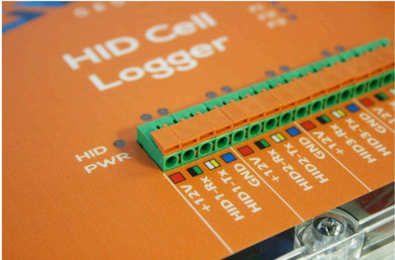
When power is switched on to the HID Cells, the LED labeled "HID PWR" will glow.
