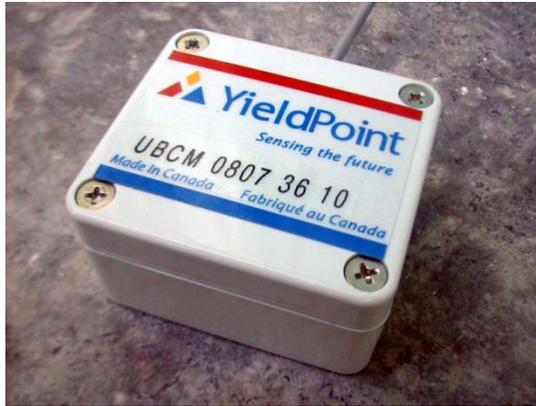
**d-TILT-SG** is a fully waterproof in-place tilt sensor based on Analog Devices' MEMS accelerometer technology. It has a wide range (0 to +/-30 arcdeg). The duty-cycle digital signal from the accelerometer is processed by the on-board micro-controller, giving typical accuracies to within 0.025arcdeg, with a resolution of 0.01arcdeg. Each sensor is individually calibrated, and temperature compensated using a digital temperature sensor that is incorporated.
