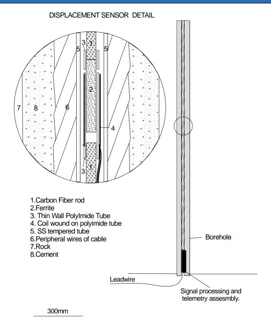
The figure above shows detail of the miniature inductive strain gauge that can be recessed into the tubular king-wire. The strain can be determined accurately *in situ* rather than translated to an instrumentation head at the end of the cable.
