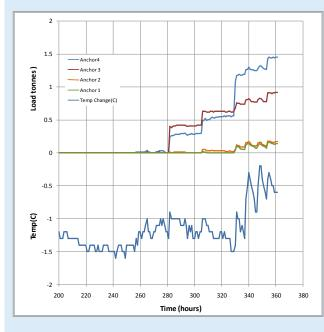
Detailed d-CABLE data recorded using a d-LOGGER.
