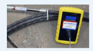
The RS485 output signal can be transmitted over 500m without amplification. Readings (one for each strain gauge) are directly in tons allowing immediate interpretation of cable load without having to enter the raw voltage data in a spreadsheet.
