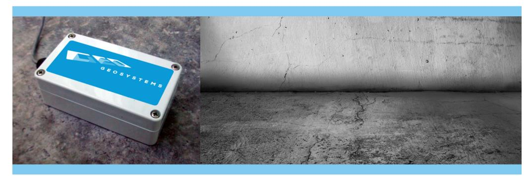
The Geosystems dual-axis tiltmeter designed for semi-permanent installation in either a borehole or surface application. The technology is based on an electrolytic tilt sensor that has a range of ±2° and an on-board digital temperature sensor. Each instrument is individually calibrated with coefficients stored in the micro-controller memory.
